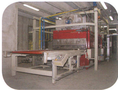
Tempera forno in piano 1360 x 3000
